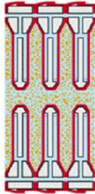
filter press full with sludge suspension
